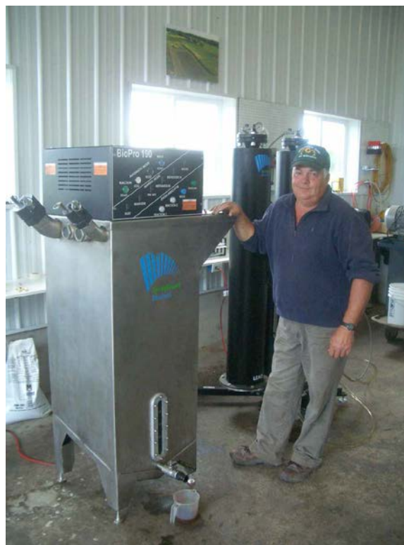
Figure 6 – Roger Rainville stands next to a BioPro 190 automated biodiesel processor at Borderview Research Farm in Alburgh, VT.
