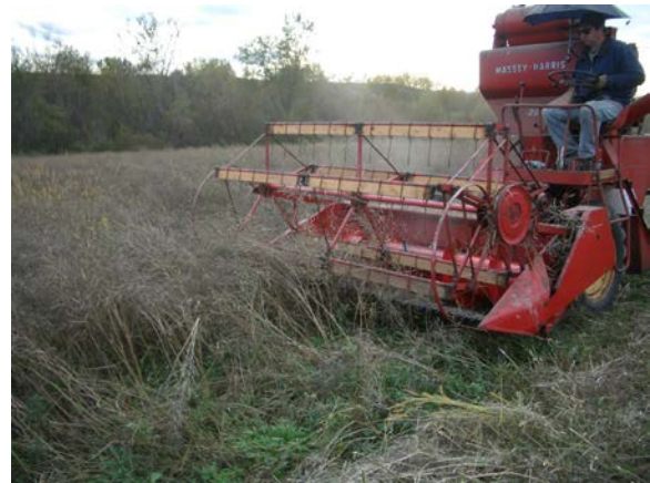
Figure 4 - Harvesting canola with a Massey-Harris SP35. In areas with few combines and where oilseeds are being trialed in small acreage, older combines like this are often the first used.
