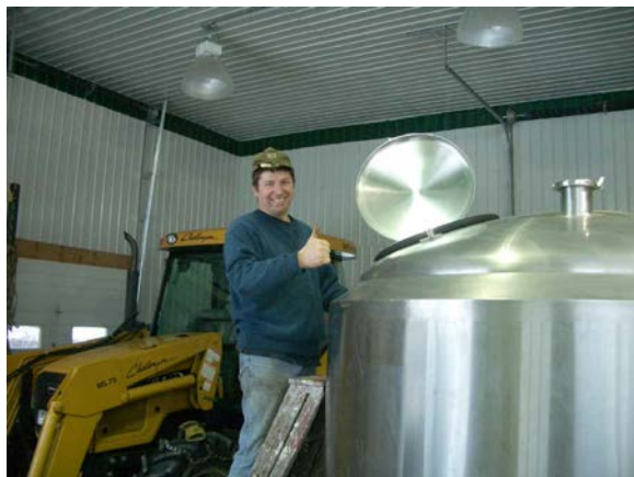
Figure 1. John Williamson at State Line Farm Biofuels in Shaftsbury, VT, checking the settling tank holding a 300 gal batch of biodiesel made on the farm.
