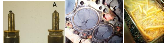
Vegetable oils have high viscosity which may lead to injector coking and eventual engine failure.
