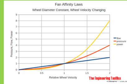
**Note:** When fan speed increases 10%, volume flow increases 10%, head increases 21%, and power consumption increases 33%.
